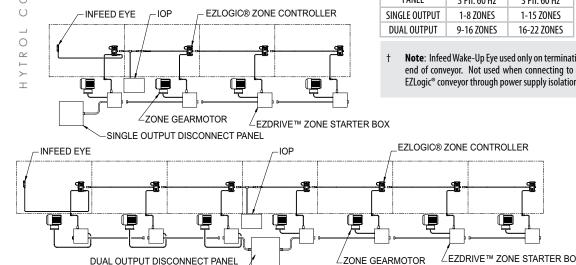
EZLOGIC° ZONE CONTROLLER-Located in each zone (Retro-Reflective). NEMA 1, 2, IP 62. UL Approved.
