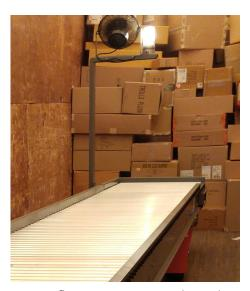
Gravity flow conveyors are dependent on truck floor elevation in order to move product. The Load-X Adjustoveyor uses a belt to move product in a fluid, controlled manner, regardless of floor elevation level. Worn bearings can cause the rollers to stop product flow.
