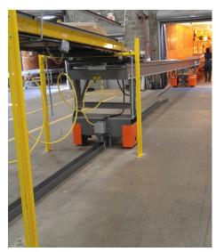
Wheels are used to roll the gravity conveyor onto the floor of the truck. Ease of movement is affected by the condition of the truck floor. The Load-X Adjustoveyor does not touch the floor of the truck, resulting in a smooth loading process irrespective of truck floor conditions.
